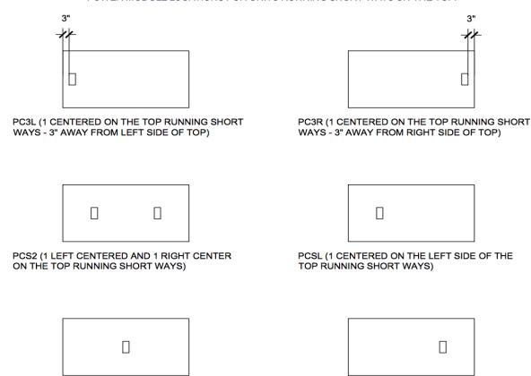
Note that power supplies cannot be placed over metal base plates, contact service@symphonytables.com to ensure that the power supply location will work with your base placement and all of the other options / accessories specified on the table.
